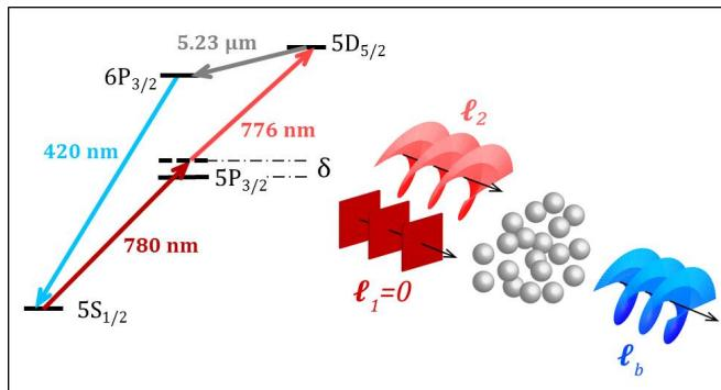
Fig. 1 :principle of vortex conversion based on the two-photon Raman excitation in rubidium.
