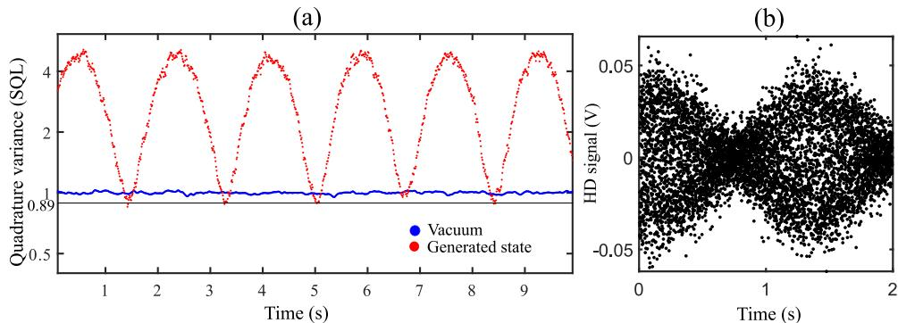
**(a)** Quadratures variances are scanned as a function of time. -2 dB squeezing below the standard quantum limit is extracted, when detection losses are taken into account. **(b)** Direct measurement of the quadratures by the homodyne detection (HD) setup.
