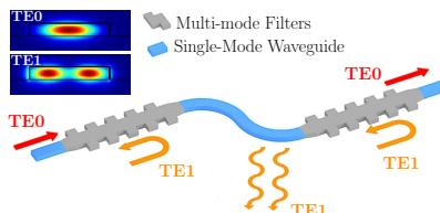
Fig. 1 : Schematic view of proposed cascaded filter. Fundamental mode ( $TE_0$ ) is back-reflected into first order mode ( $TE_1$ ). Single-mode waveguide sections separating adjacent filters radiate the back-reflected  $TE_1$  mode away, precluding coherent interaction among different stages.
