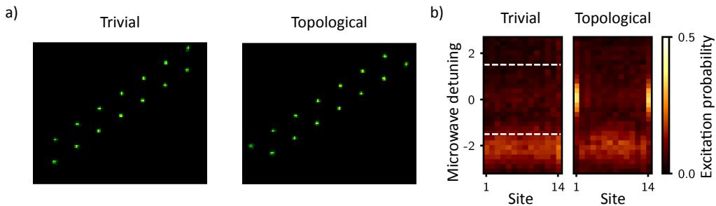
FIG. 1. Probing the single-particle signature of topology in the SSH model. (a) : Single-shot fluorescence images of the atomic arrays used to simulate the two configurations of the SSH model, the trivial and the topological ones. (b) : Site-dependent single-particle spectroscopy of the SSH chain in its two configurations. The spectroscopy in the topological case reveals the presence of edge states, signatures of topology.
