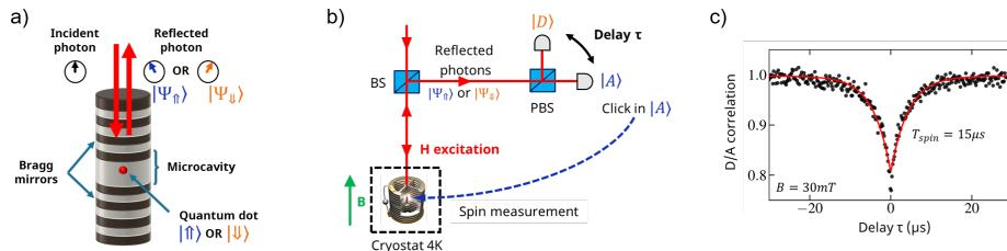
Fig. 1. (a) Polarization rotation by a micropillar cavity coupled to a charged QD. (b) Experimental cross-correlation setup. (c) Cross-correlation measurement between the A and D polarizations. The measurement back-action by a single detected photon in polarization A modifies the spin state probabilities from 50% - 50% to typically 75% - 25%. This effect lasts for a characteristic spin lifetime of 15  $\mu$ s.
