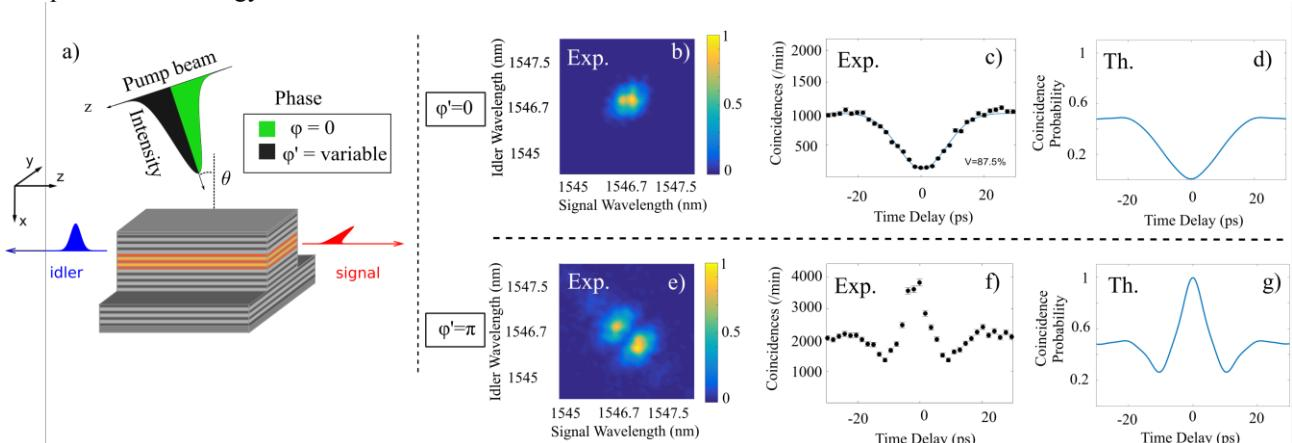
Figure 1: a) Sketch of the working principle of the device under transverse pump illumination; b-d) joint spectrum measured with a fiber spectrograph [4], corresponding experimental and numerical simulations data showing the two-photon interference in a HOM interferometer for a flat phase pump beam ( $\phi'=0$ ); e-g) joint spectrum and HOM interference for a pump beam with a pi phase shift ( $\phi'=\pi$ ).
