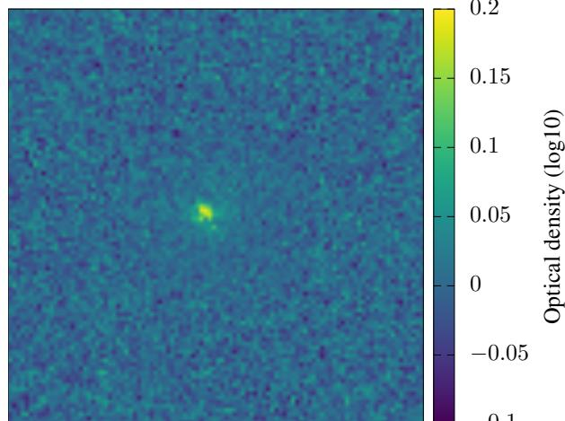
**Figure 2.** Absorption image through the multimode fiber of cold atoms captured in a micro-trap, reconstructed from the speckle. Dimension :  $100 \times 100 \text{ px} = 100 \times 100 \mu\text{m}$
