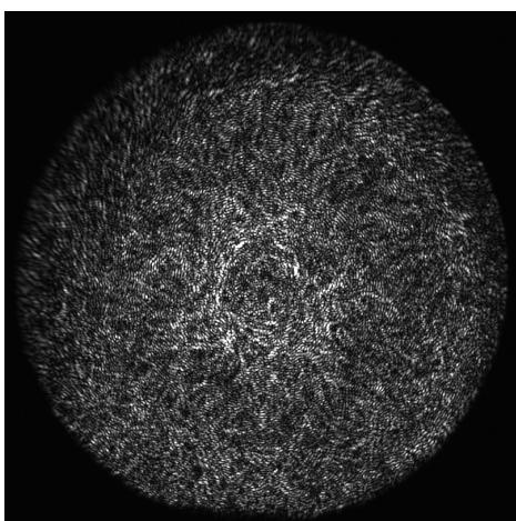
**Figure 1.** Image of light intensity outputting the multimode fiber, forming a random speckle.
