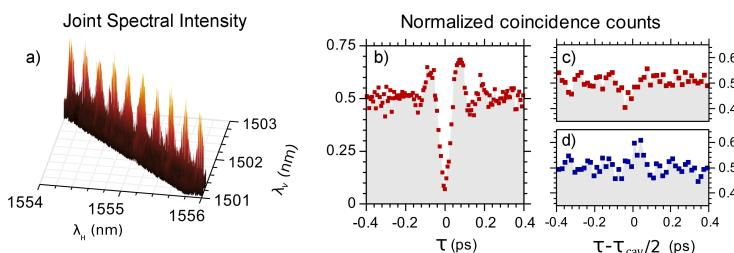
FIGURE 1 – Characterization of the biphoton state emitted by our device : measurements of the Joint Spectral Intensity (a), HOM interference at zero delay (b) and for a time delay corresponding to the half of the cavity roundtrip for two different values of the pump beam frequency (c,d)
