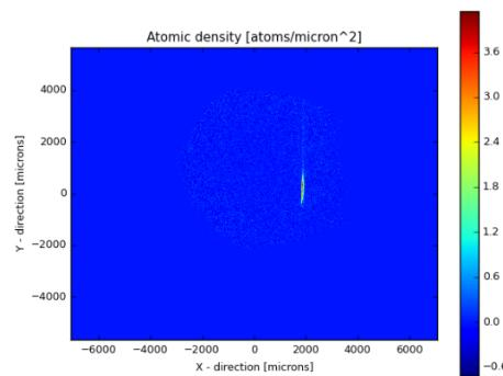
FIGURE 2: Absorption imaging of the atomic cloud after transport.
