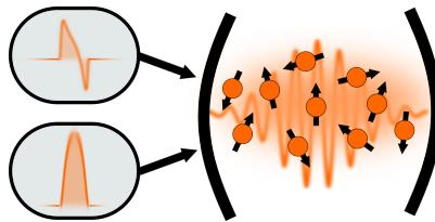
Fig. 1 : sketch of the system. The state of a spin ensemble coupled to a cavity is modified using a sequence of coherent and squeezing pulses.
