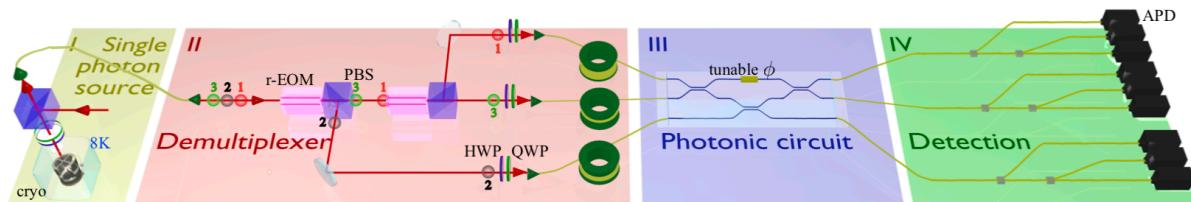
Fig. 1. **Experimental scheme of the three photon coalescence.** (I) Generation of single-photons from a QD-micropillar device under resonant fluorescence excitation. (II) Preparation of the three photons simultaneously arriving to the tritter input via active demultiplexing. (III) Photonic circuit of the tritter to perform the three photon coalescence. (IV) Detection of the quantum state of light at the tritter output.
