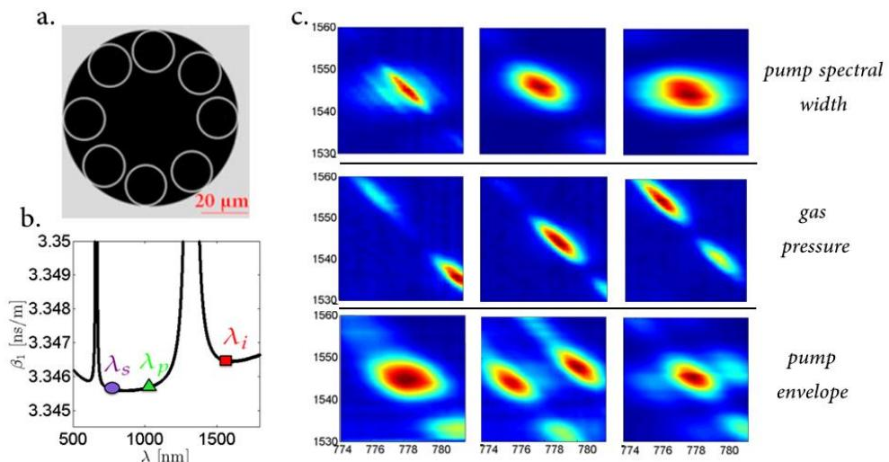
**Fig. 1** **a.** Fiber cross-section measured with an optical microscope. **b.** Simulated inverse-group velocity exhibiting a multiband profile. **c.** Measured joint-spectral intensity (JSI) of the source for different experimental parameters; The JSI are obtained using the stimulated emission tomography technique.
