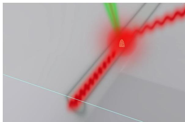
Figure 1. Schematic of a single photon coupling between well-located QDs and an optical waveguide.
